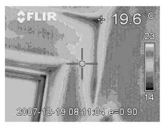
Figure 4: Thermal image of external corner of east bedroom, first floor; the dark areas show cold internal corners,
